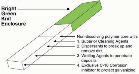
The green knit enclosure lets water pass through to contact all of the surfaces.
